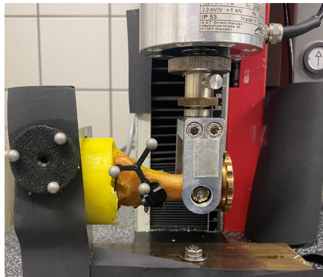
Figure 2. Test setup with potted specimen fixed on the left as cantilever beam and connected to the load cell via a hinge. Two retroreflective marker sets for optical motion tracking are attached to the fixture (left) and to the 1st metatarsal shaft (right).
